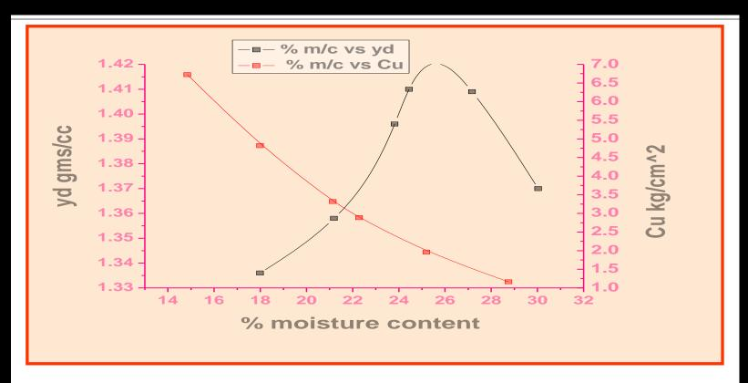
The value of  $C_u$  is determined by UCC test and the relation between % Moisture Content,  $\gamma_d$  and  $C_u$  is as shown in figure.
